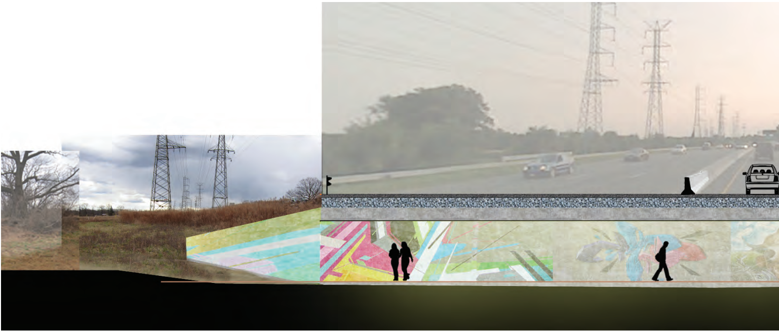
Fig. 80. Section cut through the cow tunnel under highway 1 showing an elevated boardwalk and extended art walls.
